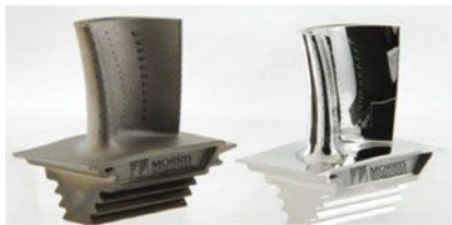
Exhibit 2: Illustration of surface finishing after EOS DMLS AM and after polishing
